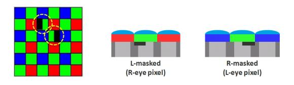
Figure 5. PD Pixel Structure inside Image Sensor
